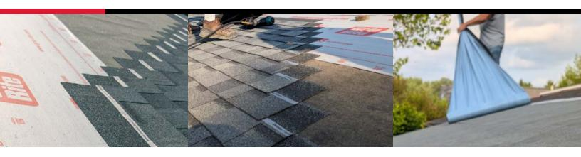
Grip-Rite® Eave & Valley Protector provides additional protection against roof damage caused by ice and water. This 53-mil self-adhesive membrane is composed of elastomeric bitumen with glass mat reinforcement to create a non-slip surface. Install beneath shingles, and along areas where water may collect. The easy-to-remove silicone treated split-back release sheet makes it easy to install and quickly provides protection to the most vulnerable areas of the roof.
