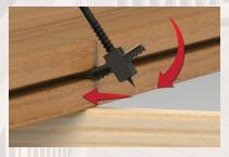
1 On the outside edge of the installed starter board, hold the clip at an angle and insert the compression fit tabs.<sup>†</sup> Then rotate and push the Grip-Bite™ razor teeth into the groove. The clip will now stand securely.
