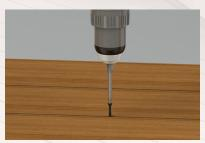
5. With the new board held firmly in place, fully tighten down the screws of each Grip-Rite Ninja clip. Set the drill to 1/3 of the Max torque. If your drill has the option of a clutch mode it is recommended you use that. Impact Drills should not be used with Grip-Rite Ninja Clip.
