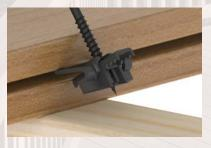
On the outside edge of the installed starter board, hold the clip at an angle and insert the precision fit tabs.<sup>†</sup> Then rotate and push the Grip-Bite™ razor teeth into the groove. The clip will now stand securely.
